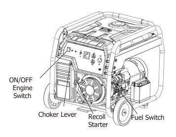
Turn the Engine Switch to "ON" position.
