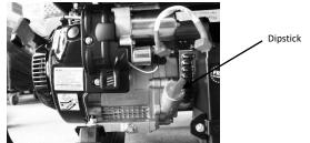
MOTICE Improper treatment of generator could damage it and shorten its life. DO NOT attempt crank or start the engine before it has been properly serviced with the recommended oil. This could result in an engine failure.
