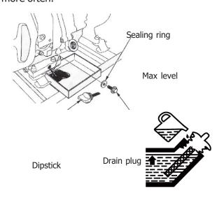
⚠ CAUTION Hot oil may cause burns. Allow engine to cool before draining oil. Avoid prolonged or repeated skin exposure with used oil. Thoroughly wash exposed areas with soap.
