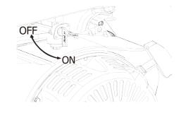
Move engine choke lever to the OFF position
